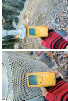
Measure flammable atmospheres before starting hot work.
